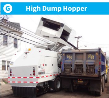
G High Dump Hopper Variable dump height hopper (up to 12' 2" high) with 54" extra-long dump door easily reaches most dump trucks.
