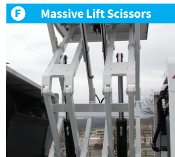
F Massive Lift Scissors Massive double "X" style lift scissors & 4-corner hopper lift ensure exceptional hopper stability when dumping wet, unbalanced, or sticky debris.
