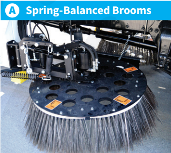
A Spring-Balanced Brooms Spring-balanced, free-floating main & gutter brooms automatically apply correct surface pressure for maximum broom wear life. In-cab gutter broom electric tilt is standard.
