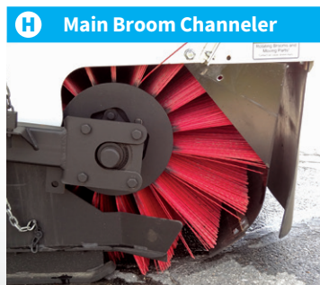
H Main Broom Channeler Main broom channeler (optional) effectively sweeps large quantities or bulky & light debris (leaves/pine straw). Self-adjusting as main broom wears.
