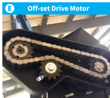
E Off-set Drive Motor Off-set hydraulic elevator drive motor is protected against shock loading.
