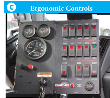
C Ergonomic Controls Vertically-mounted control panel is 6-way adjustable for easy & ergonomic viewing. One-touch sweeping allows for operator to preset functions. Brooms raise automatically in reverse.
