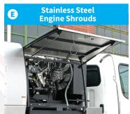
Stainless steel engine shrouds are compact, protective & noise reducing. Gull wing design makes it easier & faster to service power plant without raising an interconnected hopper/shroud assembly.
