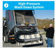
Optional High-Pressure Wash Down System with 50' hose reel & spray wand allow separator screens & hopper to be cleaned at any time which can improve vacuum performance.
