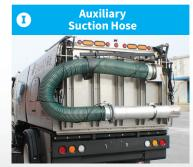
Optional rear-mounted 10' Auxiliary Suction Hose with 4' aluminum tube helps clean storm drains.
